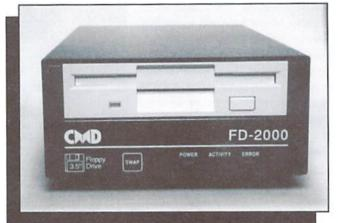
drive mechanism, and is the traditional IBM clone beige color. The front panel contains 1 switch and 3 LEDs in addition to the customary manufacturer logo and drive model number. The LEDs are labeled "Power", "Activity", and "Error". Turning the unit around, we see the back of the unit is pretty simplistic as well. Two serial bus connectors are provided, as is a connector for the power supply and a power switch.
