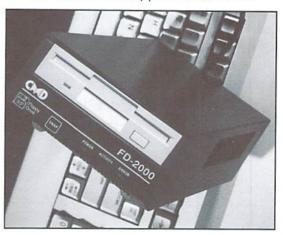
be careful, as the Phillips screws holding it in are of aluminum, and can strip easily, rendering installation much harder.) Since CMD has made it possible for users to do the installation themselves, a switch to a screw that is more forgiving to typical user tools would be beneficial.
